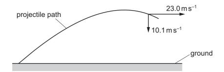
At a certain time, the projectile has a horizontal velocity of  $23.0\,\mathrm{m\,s^{-1}}$  and a vertical velocity of  $-10.1\,\mathrm{m\,s^{-1}}$ .
