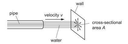
When the jet of water hits the wall, it has horizontal velocity *v* and cross-sectional area *A*.
