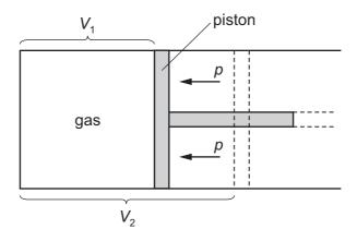
Initially, the gas has a volume  $V_1$  and is in equilibrium with the external pressure p. The gas is then heated slowly so that it expands at constant pressure, pushing the piston back until the volume of the gas has increased to  $V_2$ .
