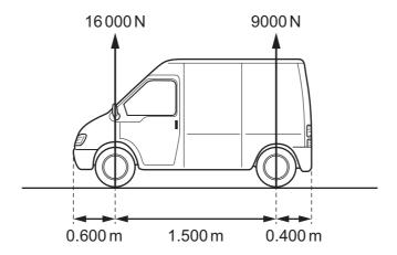
The van is 2.50 m long with the wheels at a distance of 0.600 m from the front of the van and 0.400 m from the rear of the van.
