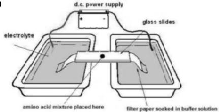
power supply (idea of complete circuit) electrolyte/buffer solution gel/filter paper/absorbent paper (amino acid) sample/mixture [centre of plate]
