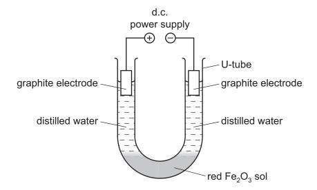
(b) The student placed a few cm³ of the sol at the bottom of the U-tube and poured 10 cm³ of distilled water into each side of the U-tube, without disturbing the sol. The two layers of distilled water were colourless at the beginning of the experiment. Graphite electrodes were inserted and a current was passed. After 30 minutes a difference was noted between the distilled water in the two sides of the U-tube.
