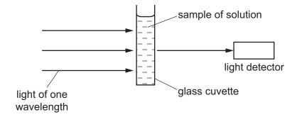
(a) (i) A chemist placed distilled water in the glass cuvette. This was then put into the spectrophotometer and a reading taken.
