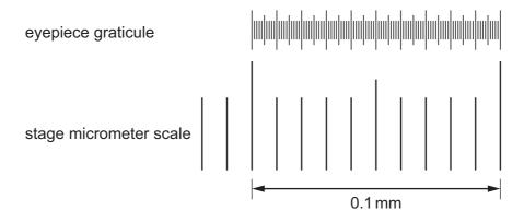
How is the value, in  $\mu m$ , of one eyepiece graticule unit calculated?
