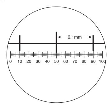
Using the same magnification, a chloroplast is measured and found to be 4 eyepiece graticule divisions long.
