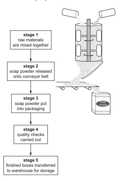
Each of these stages uses machinery controlled by a production worker.
