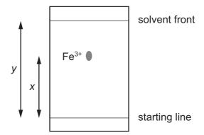
To make the spot containing  $Fe^{3+}$ (aq) more visible, the paper is sprayed with aqueous sodium hydroxide so that a precipitate of iron(III) hydroxide forms.
