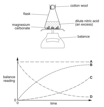
A graph of the balance reading against time was plotted. Which curve was obtained?
