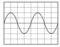
The time-base on the oscilloscope is set to 4 ms/cm.
