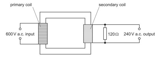
What is the power dissipated in the resistor and what is the current in the primary coil?
