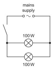
How much electrical energy is supplied by the mains when the switch is closed for 36 minutes?
