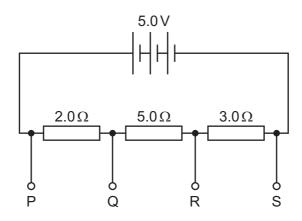
Between which pair of terminals is there a potential difference of 1.5 V?
