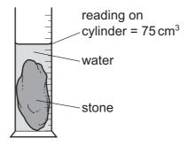
The volume of water in the cylinder before adding the stone is 15 cm<sup>3</sup> and the stone has a mass of 90 g.
