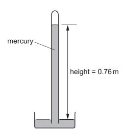
What is the pressure exerted by the atmosphere when the height of the mercury in the simple barometer is 0.57 m?
