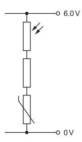
Under which conditions is the voltage across the fixed resistor the greatest?
