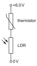
The thermistor has a resistance of  $6000\,\Omega$  in a cold room and  $1000\,\Omega$  in a warm room. The LDR has a resistance of  $2000\,\Omega$  in dim light and  $500\,\Omega$  in bright light.
