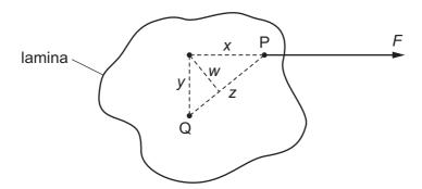
The lamina is free to rotate about point Q.
