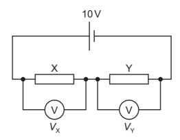
What is the difference  $V_Y - V_X$  of the voltages shown on the voltmeters?
