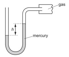
The pressure of the atmosphere is  $p_0$  and the density of mercury is  $\rho$ .
