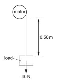
The load weighs 40 N. The power of the motor is 20 W and the system is 25% efficient.
