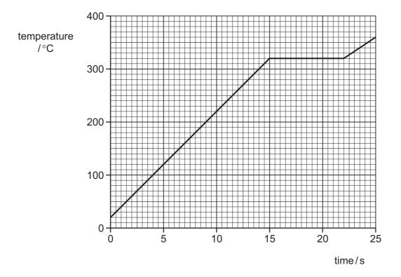
The power of the heater is 320 W.
