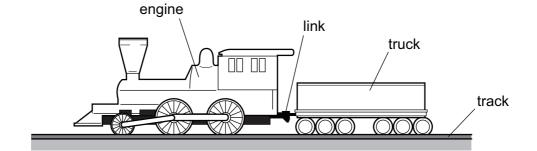
The link between the engine and the truck breaks. The driving force on the engine remains constant.
