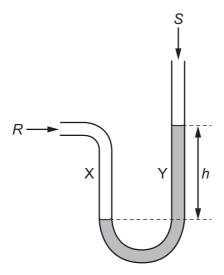
Side X is connected to a gas supply of pressure *R*. Side Y is open to the atmosphere at pressure *S*.
