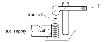
What does the end P do when the switch is closed?
