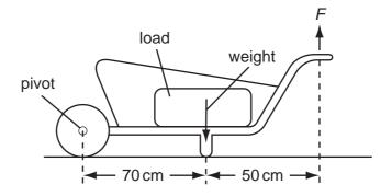
What is the size of force F needed just to lift the loaded wheelbarrow?
