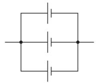
What is an advantage of this arrangement of cells?
