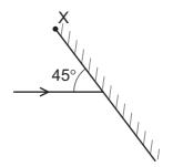
The mirror is rotated until the light is reflected back along its original path.
