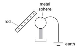
The earth connection is removed and then the rod is removed.
