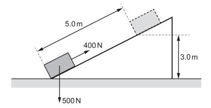
Part of the work done increases the gravitational potential energy E of the crate and the rest is work done W against friction.
