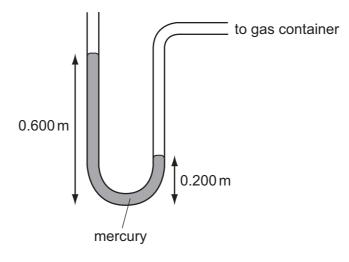
The density of mercury is  $13600 \text{ kg/m}^3$ . The gravitational field strength g is 10 N/kg.
