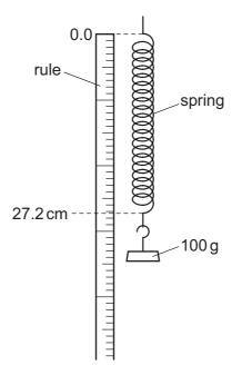
The 100 g mass is replaced with a 600 g mass. The length of the spring is now 89.7 cm. The spring has not reached the limit of proportionality.
