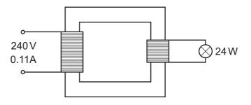
The input current to the transformer is 0.11A and the input voltage is 240 V. The useful output power of the transformer is 24 W.
