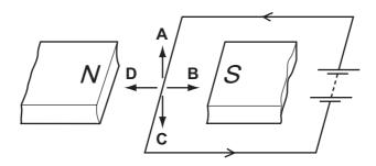
**34** A simple d.c. motor consists of a coil that rotates between the poles of a permanent magnet. The turning effect is increased by winding the coil on a metal cylinder.
