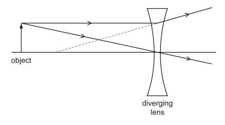
**23** The ray diagram shows two rays from a point on an object placed in front of a diverging (concave) lens.
