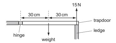
When the trapdoor is closed, the ledge exerts an upward force of 15 N on the trapdoor. The gravitational field strength is  $10\,\text{N/kg}$ .
