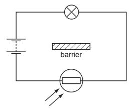
When low intensity light falls on the LDR, the lamp glows dimly.
