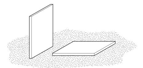
After a few hours, the vertical tile has started to sink into the soft earth, but the horizontal one has not.
