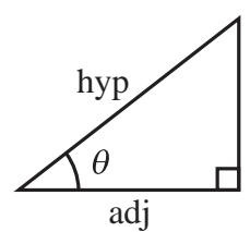
$$\begin{aligned} \text{adj} &= \text{hyp} \times \cos \theta \\ \text{opp} &= \text{hyp} \times \sin \theta \end{aligned}$$
