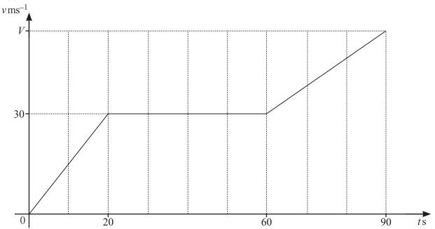
The diagram shows the velocity–time graph of a particle P that travels 2775 m in 90 s, reaching a final velocity of  $V \, \mathrm{ms}^{-1}$ .
