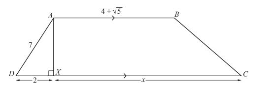
The diagram shows a trapezium *ABCD* in which AD = 7 cm and  $AB = (4 + \sqrt{5})\text{ cm}$ . *AX* is perpendicular to *DC* with DX = 2 cm and XC = x cm. Given that the area of trapezium *ABCD* is  $15(\sqrt{5} + 2)\text{ cm}^2$ , obtain an expression for x in the form  $a + b\sqrt{5}$ , where a and b are integers. [6]
