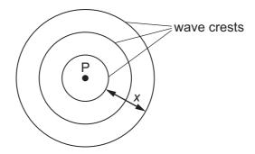
Three wave crests are produced every six seconds. Distance x is equal to 40 cm.
