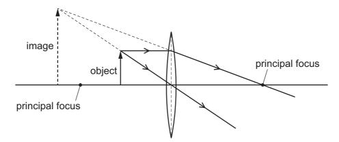
The object is moved to the right, closer to the lens.
