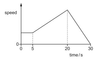
The car travels 60 m while it brakes to a stop.
