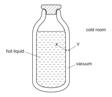
How is energy transferred through the vacuum between X and Y?
