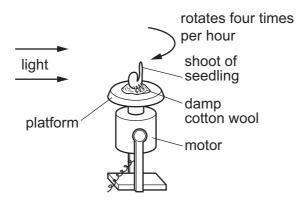
The platform is rotated four times every hour, for two days.
