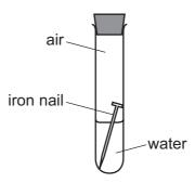
Which change in the air in the test-tube occurs as the iron nail rusts?
