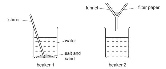
The contents of beaker 1 are stirred and then poured into the funnel above beaker 2.
