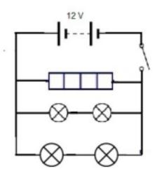
sidelamps remain in series with each other and each pair in parallel with the battery ; heater, sidelamps, headlamps all in parallel ;
