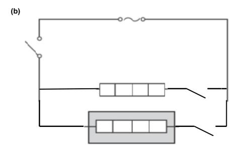
switches in both heater branches (can be either side of heater) ; rest of circuit completed properly ;
