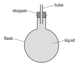
A Bunsen burner is used to heat the liquid in the flask. Some liquid flows out of the top of the tube.
