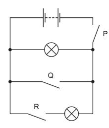
Which switches must be closed so that both lamps light?
