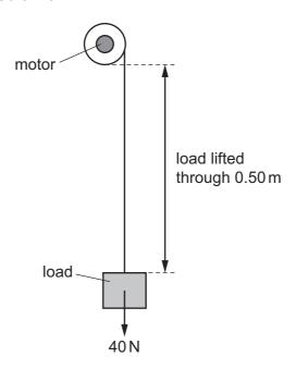
The power of the motor is 40 W and the system is 20% efficient.
