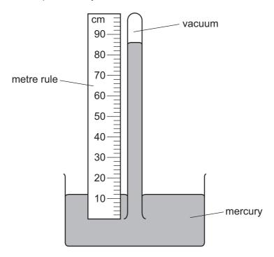
Which length is used to find the value of atmospheric pressure?
