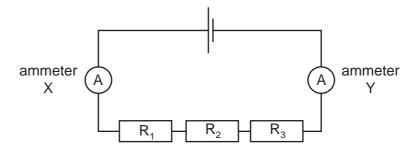
Which of the ammeters will show the current in resistor R<sub>2</sub>?
