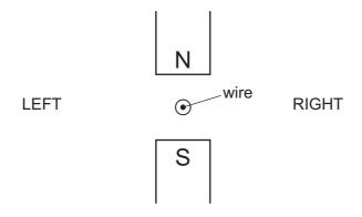
The wire is moved and a current is induced upwards, out of the paper.
