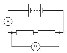
The voltmeter reading is 2.2 V and the ammeter reading is 0.25 A.
