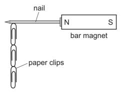
The bar magnet is then removed and the number of paper clips remaining attached to the nail is recorded. Each nail is tested individually.
