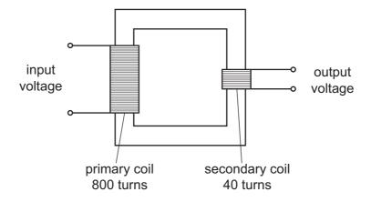
The input voltage is 240 V.
