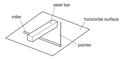
The roller rests on a horizontal surface and the steel bar rests on top of the roller.
