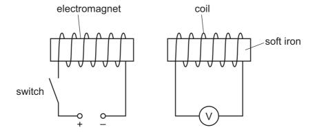
The switch is closed. The electromagnet magnetises quickly.
