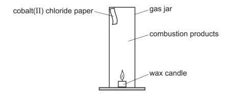
After a short time, the oxygen in the jar is used up and the candle flame goes out.
