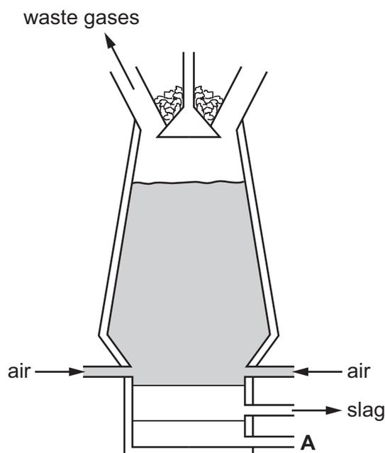
(i) Coke and iron ore are added at the top of the blast furnace.
