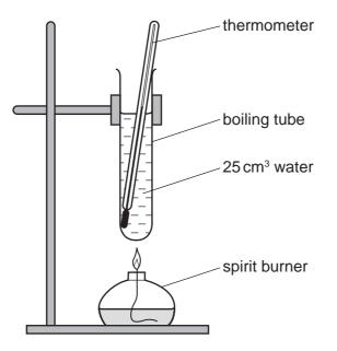
(a) Some methanol was put into the burner. The initial temperature of the water was measured. The burner was lit and allowed to burn for one minute. The flame was extinguished and the final temperature of the water was measured. The experiment was repeated with ethanol, propanol and butanol.
