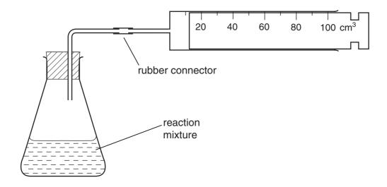
By using a measuring cylinder,  $20\,\mathrm{cm^3}$  of hydrogen peroxide was placed in the flask and 0.8 g of the catalyst, manganese(IV) oxide was added. The bung was replaced and the gas collected was measured at 1 minute intervals. The results were plotted on the grid (opposite).
