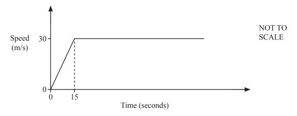
The car starts from rest and accelerates at a uniform rate for 15 seconds before reaching a constant speed of  $30 \,\mathrm{m/s}$ .
