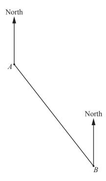
Measure the bearing of point B from point A.
