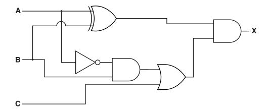
(a) Complete the truth table for the given logic circuit.
