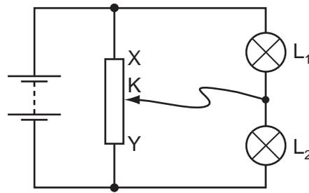
The contact K is halfway between X and Y and the lamps are equally bright.
