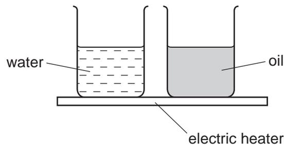
The temperature of the water and the temperature of the oil increase constantly. The rise in temperature of the oil is much greater than that of the water.
