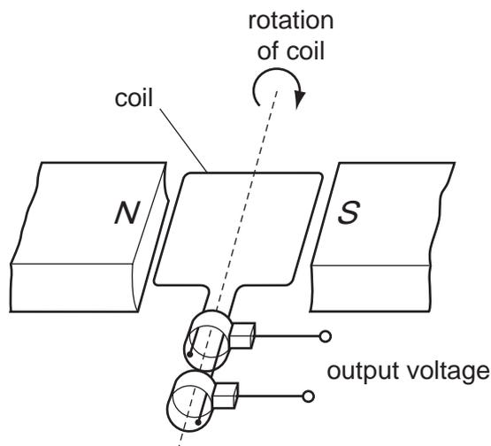
With the coil in the position shown, the output voltage is +10V.
