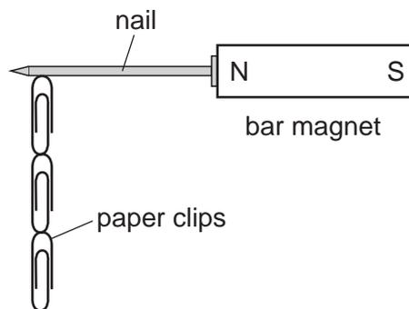
One of the nails is placed against a bar magnet and the number of paper clips which the nail can support is recorded. The bar magnet is then removed and the number of paper clips remaining attached to the nail is recorded. Each nail is tested in turn.
