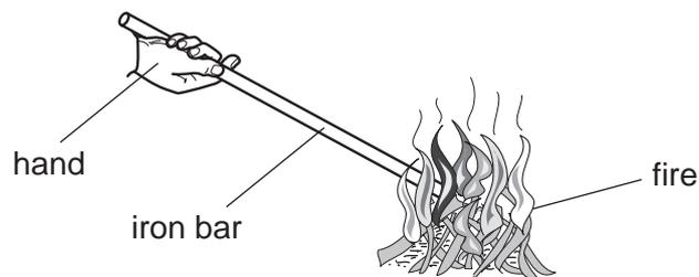
How has the heat travelled along the iron bar?
